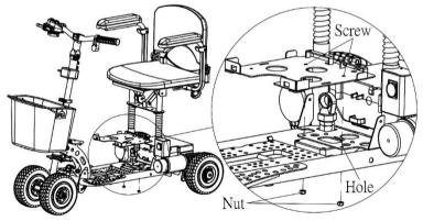
Assemble the battery tray as illustrated. Insert the screws and tighten the nuts. When using a lithium battery it is recommended that you place your lithium battery on rear tray of the scooter and your SLA battery on the front tray.
