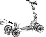
• Press the lock tab of connector and pull out to disconnect the connector as per illustration.
