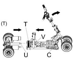
• The pin will click when inserted correctly. You must check that the pin has locked into position.
