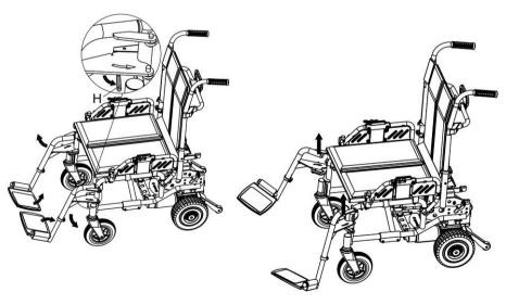
• Turn the footrest outward direction and lift up for dis-assembly.
