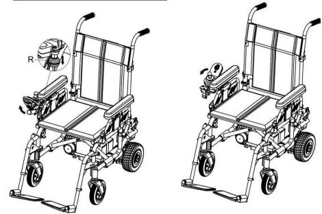
• The joystick can be swung rearwards by pulling the knob "R" rotating the joystick back alongside the armrest.
