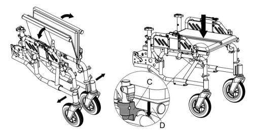
Open the backrest per illustration and insert into the corresponding hole and tighten the clamp G.
