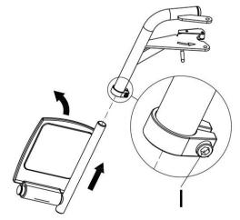
• The height of footrest can be adjusted with bolt "I".
