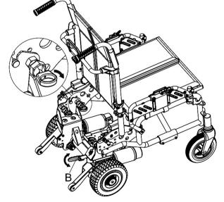
• Both side lock pins must be securely in position.
