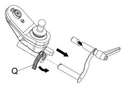
Assemble the attendant control per illustration and plug the cable P2.
