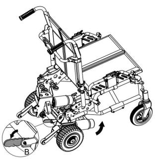
• Push down on lever B to lift the motor upwards to the horizontal position and hold it. Use the other hand to turn all 4 frame locking pins clockwise and check that they lock into positions. Lever B may need pushing down firmly to allow all pins to fully engaged.
