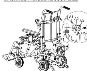
The backrest angle can be adjusted by unscrewing F1 and pulling F2 out, then insert by choosing different angles for A1, A2 or A3.
