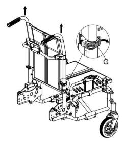
• Remove the backrest and fold per arrow direction as illustrated.
