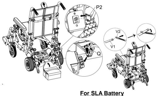
Install the battery into the tray and fasten it securely. Tighten the battery strap as illustrated.
