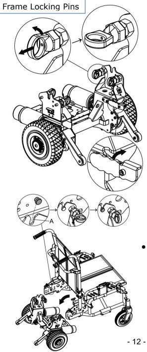
• Pull the frame locking pins on both sides and turn them anticlockwise per illustration.
