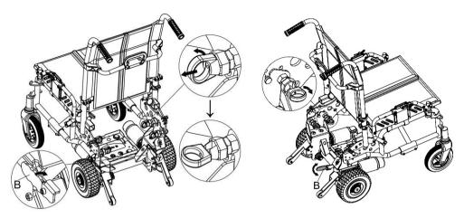
• Use one foot to press the lever "B" and use both hands to hold the handles of backrest to let guide pins release from side plates and move the chair out of motor drive mount.
