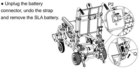
• Pull out the cable connector P2 as indicated. (Refer to P.33)
