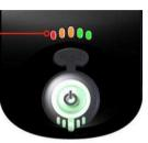
The battery gauge LEDs are also used to display charging information. See section 7.2 Battery charging for more details.
