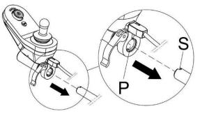
• Tighten clamp correctly and be sure that joystick is securely mounted.
