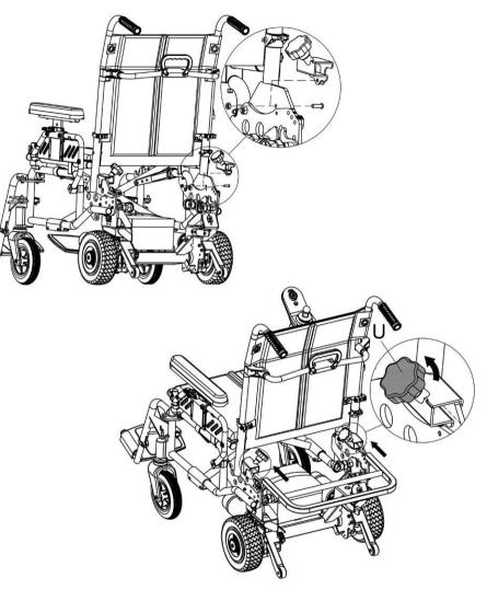
Assemble the luggage frame per illustration and tighten bolt "U". **NOTE:**
