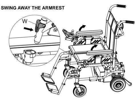
• The armrest can be lifted up by pushing "W" and can be locked by pressing down.
